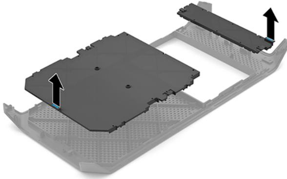
4. Install the new dust filters in the same locations as the previous dust filters.
