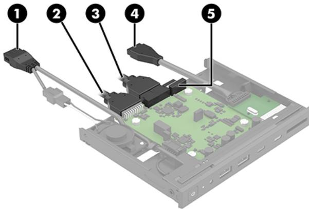
8. Release the I/O assembly by lifting up on the drive release bar **(1)**.
