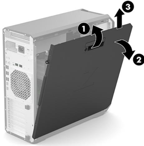
Reverse this procedure to install the access panel.
